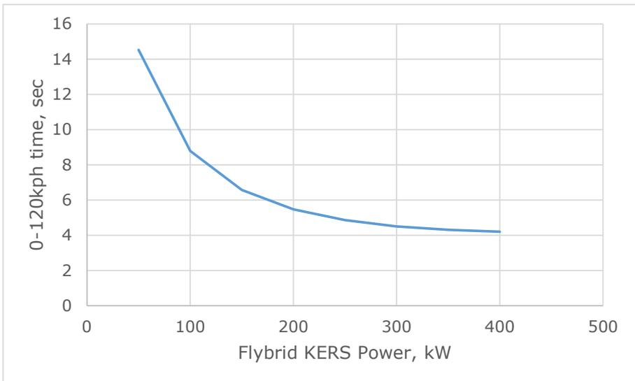
**Figure 10 – 0-120kph acceleration time for different KERS power with 1100kJ energy**
