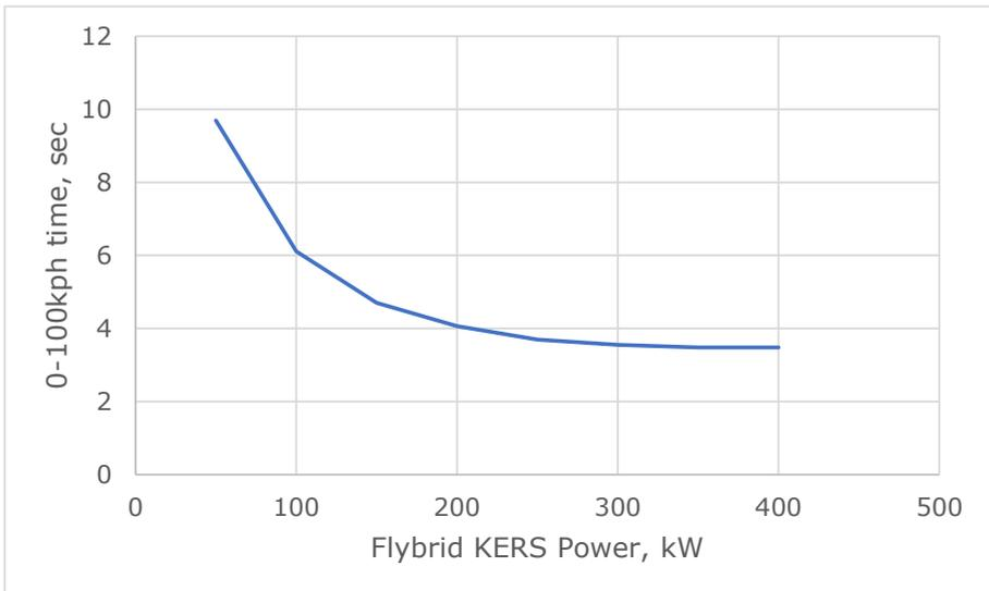
**Figure 8 – 0-100kph acceleration time for different KERS power with 800kJ energy**
