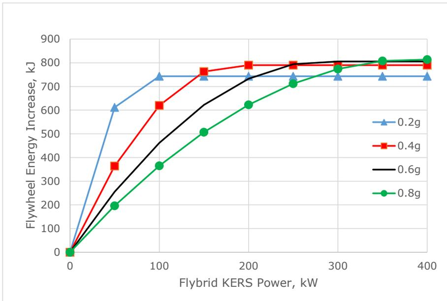
**Figure 6 – 120-0kph Energy Stored at different decelerations rates**
