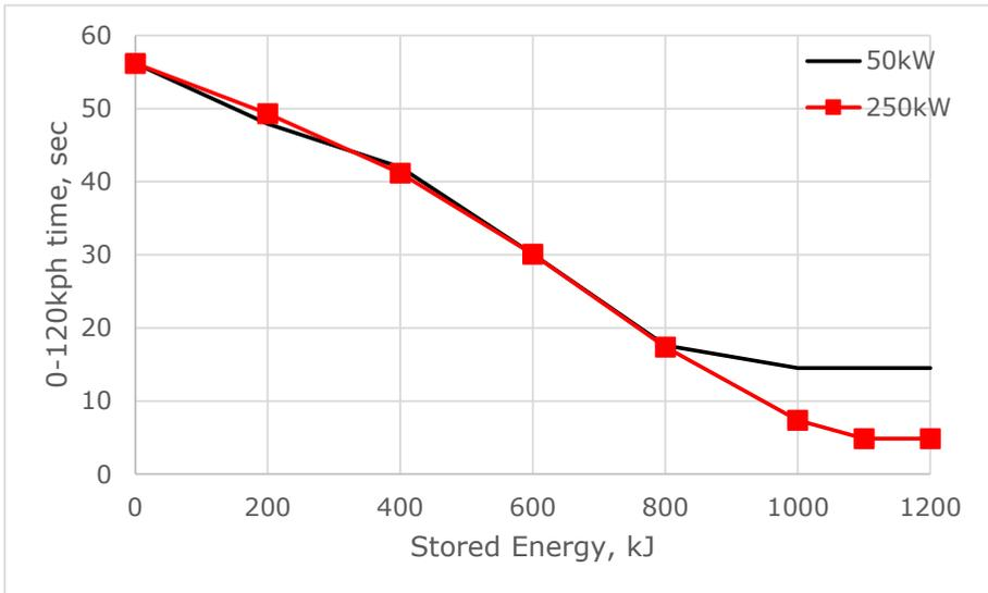
**Figure 9 – 0-120kph acceleration time for different KERS power and energy**
