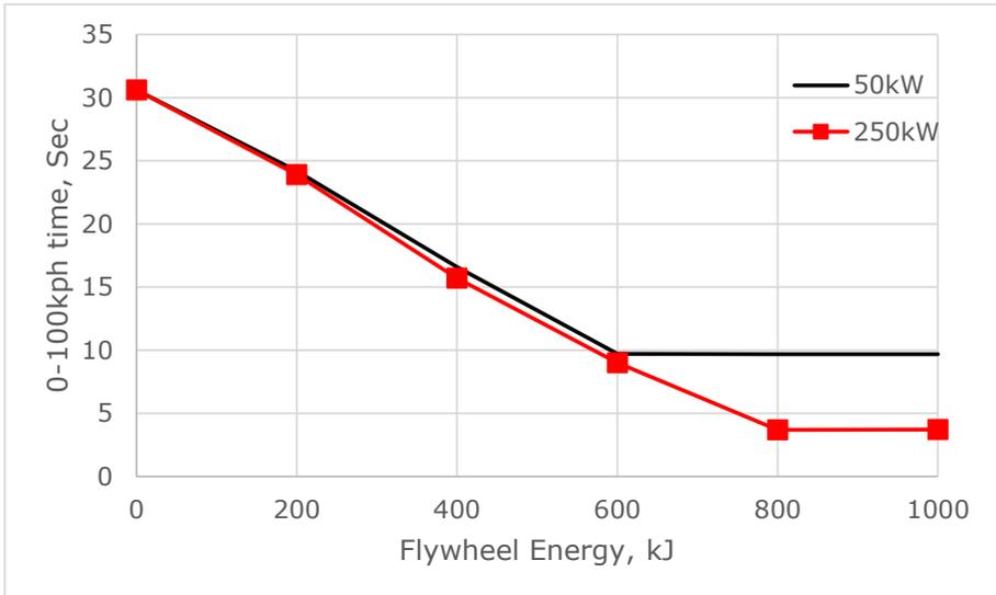
**Figure 7 – 0-100kph acceleration time for different KERS power and energy**
