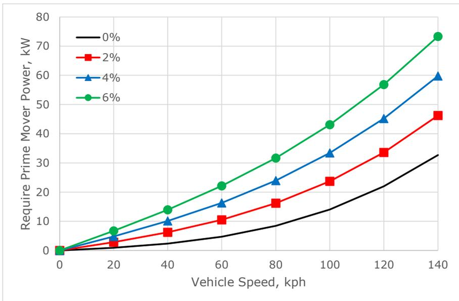
**Figure 11 – terminal vehicle speed with different road gradients and prime mover power**
