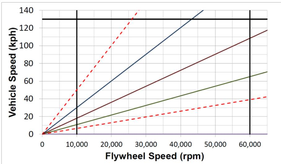
**Figure 3 shows a typical ratio spread for a 3 clutch CFT**
