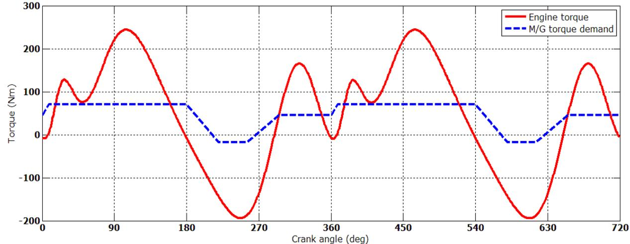
\* To give a clear view of the M/G torque, the torque demand curve is mirrored around x-axis.
