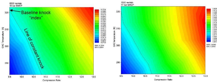
**Figure 11. The variation of knock intensity to compression ratio and CAC outlet temperature at two full load conditions**
