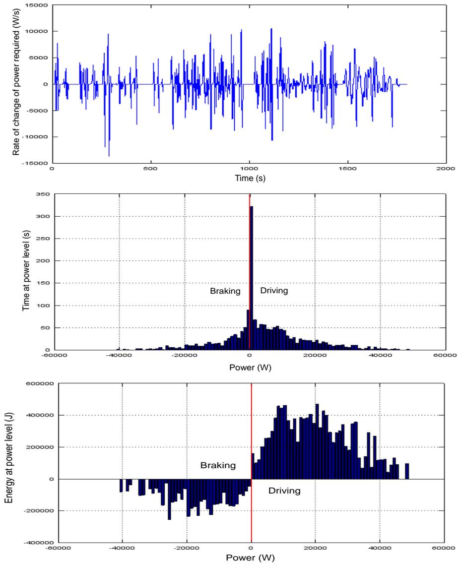
**Figure 2. Example results from the vehicle energetic analysis – looking at the WLTP with different parameters**
