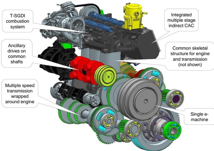
**Figure 9. An initial design layout for the chosen InPaCT concept**
