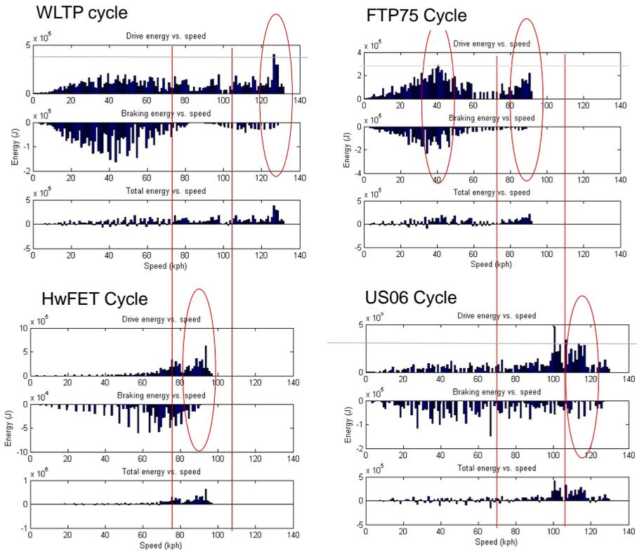
**Figure 3. Example results from the vehicle energetic analysis – looking at the ideal points for efficient powertrain operation (circled in red) over different test cycles**
