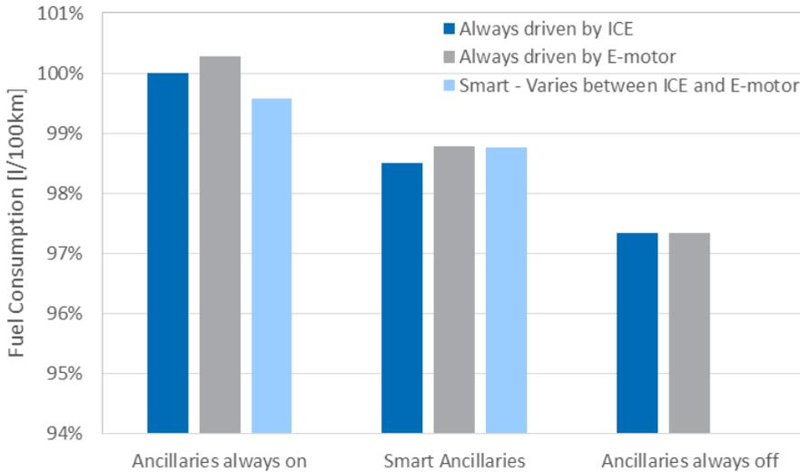
**Figure 10. Relative fuel consumption values for different configurations of ancillary control over the NEDC**
